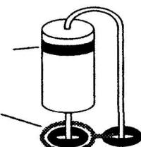
[ ] D2 1N4148 -upright If a Diode is mounted upright, there is a circle as an outline on the PCB. Mount the diode with its body inside the circle, the band (cathode) agt the upper side (see picture left!)
