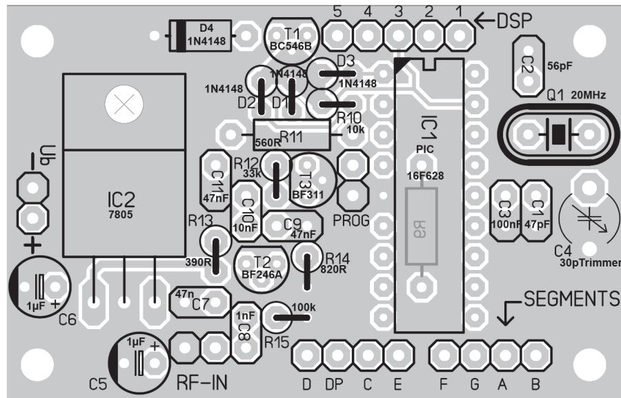
Use the PCB as shown in the picture to get some orientation. Don't install the connectors now, this will be done later on.
