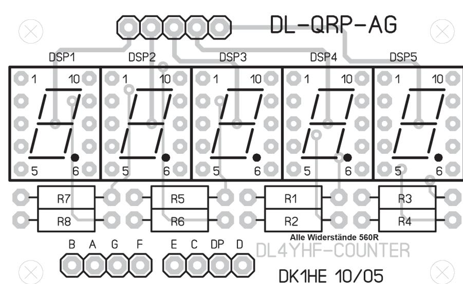
the decimal point at the right place. Look at the Picture above to see how they must be installed. Press each Display firmly against the PCB and solder 1 pin at a corner first. Check if it is realy sitting flat on the PCB and solder a pin diagonal opposite. Check again if the display is flat on the PCB. If not, reheat and press the display down to the PCB. If it is ok, solder all remaining PINs. Same procedure for all 5 Displays.
